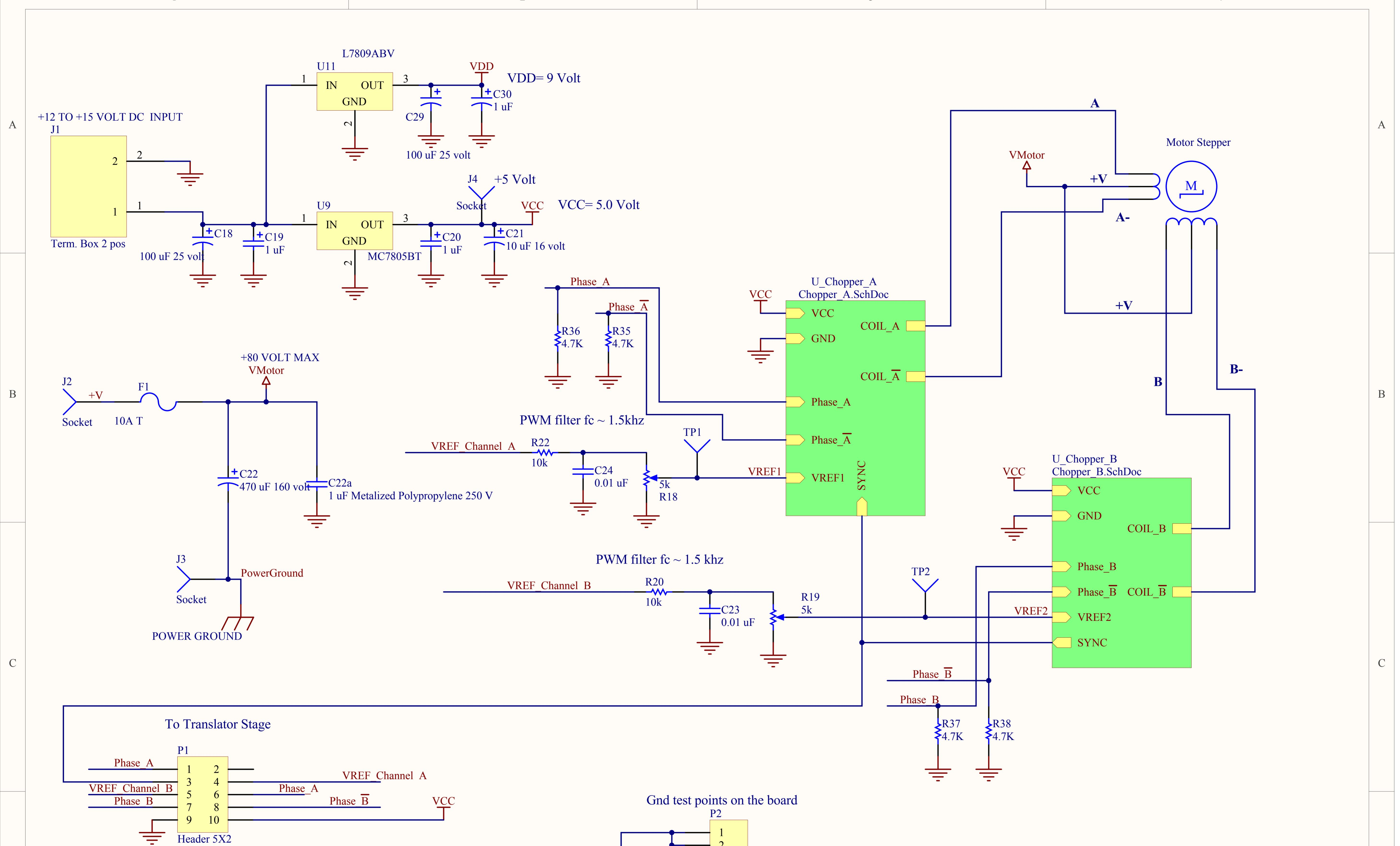
R34, R35, R36, R37 (4.7K) pull-down resistors are required in order to avoid the output transistors to turn on during power up or in case the translator circuit is not connected to the board, and during the microcontroller initialization stage after reset or power up. +12 volt must be present before powering up the +Vmotor power supply.
