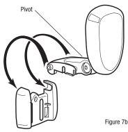
Attaching the Large Transducer Assembly to the Bracket
