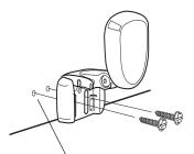
Use Marine Grade Silicone Sealant to Seal Drilled Holes
