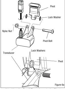
Attaching the Small Transducer to the Pivot
