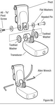
Attaching the Large (XT Series) Transducer to the Pivot
