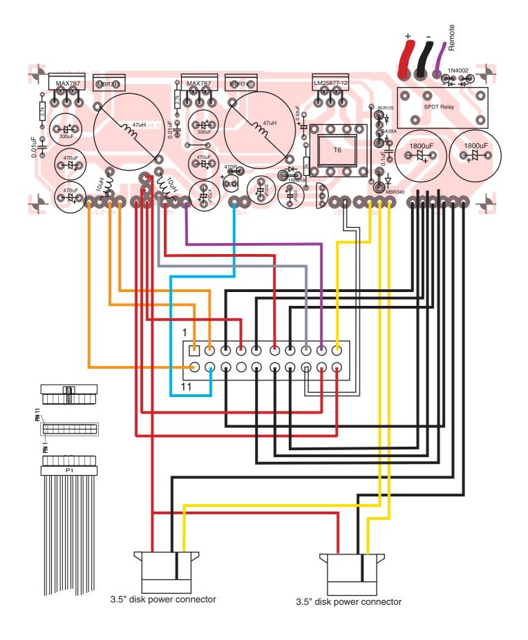
Note: This arrangement is only capable of supplying 5A at 5V and 5A at 3.3V Please ensure that current consumption is within these limits.
