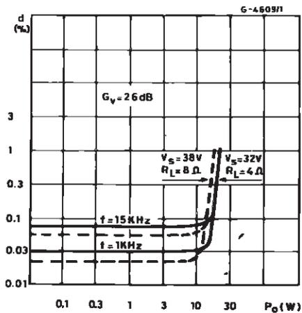
Figure 5 : Two Tone CCIF Intremodulation Distortion
