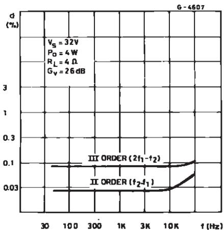
Figure 6 : Large Signal Frequency Response
