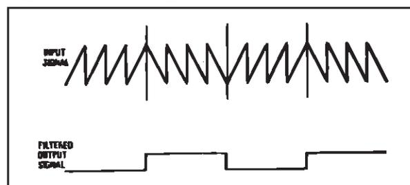
In the case of the sawtooth in Figure 25 the mean level was increased by the TIM distortion, for a sawtooth in the other direction the opposite is true. The result is an AC signal at the output whose peak-to-peak value is the TIM voltage, which can be measured easily with an oscilloscope. If the peak-to-peak value of the signal and the peak-to-peak of the inverting sawtooth are measured, the TIM can be found very simply from:
