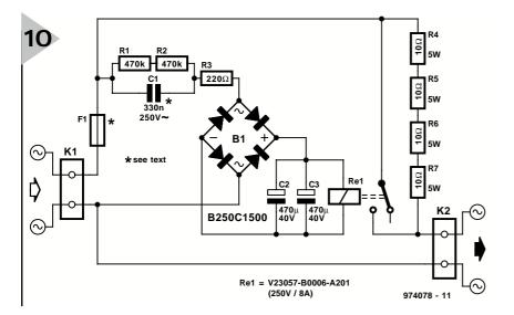
Figure 10. The mains-on delay ensures that the switch-on current remains within certain limit. Two of these delays are required for each Titan 2000.
