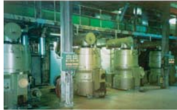
Pelleting plant with 4 presses
