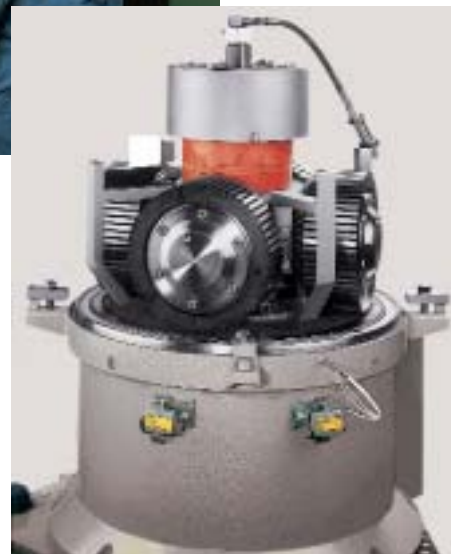
Driven pan grinder rollers for products with extreme slipping properties
