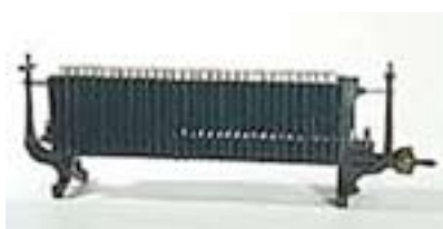
Left: Gülcher's thermopile: c 1898. This example is in the History Museum of the University of Pavia in Lombardy, Italy.
